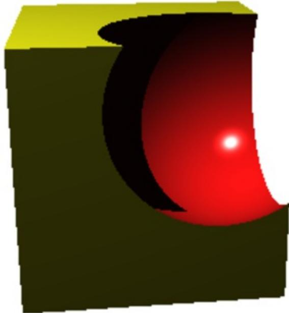
*Difference* preserves only the portion of the first shape where it's not overlapped by the others. Here's the difference between the original cube and sphere, effectively carving the sphere out of the cube.
